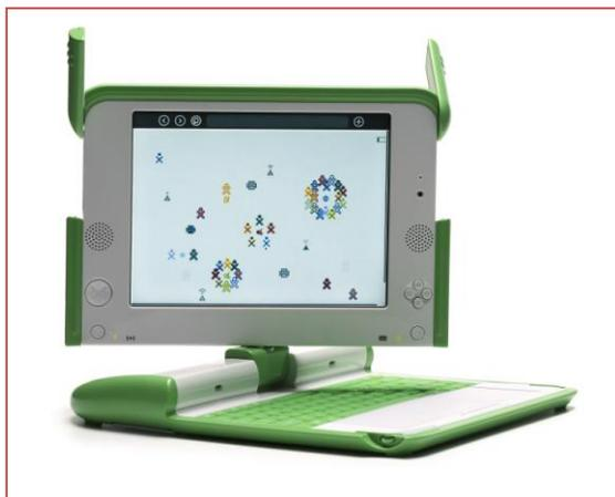
The resulting machines (pictured) were relatively impressive feats in hardware. They included a durable plastic shell and no sensitive moving parts along with a dust and water-resistant design that would keep them intact in the face of prolonged abuse and rough environments. Their speed, while limited, was unimportant because they featured a custom-designed Linux-based operating
